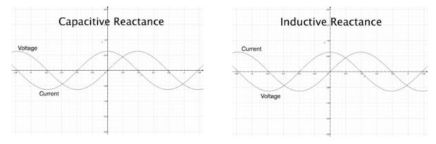
designed impedance, the antenna presents 50-ohm, non-reactive load only at its natural resonant frequencies. At other frequencies, it will exhibit capacitive or inductive reactance, causing it to have an impedance other than 50 ohms.
