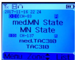
Typical radio display where A Channel is the TX channel
